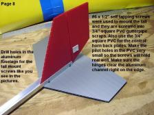
The control horns are made from PVC gutterpipe and are 1\* high by 1\* long by 1/2\* wide base. Clean the parts and use drops of CA to hold them in place so adding the screw seasier. Extra screws that come with Dave Brown engine mounts make perfect control horn screws.
