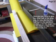
You are almost done! Trim the trailing edge flush and then cut out a wing wrap from 2mm Coroplast. Make it 17" x 4" with the flutes going in the 4" direction.
